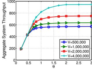
Fig. 5: Total system throughput versus the multiplier  $\theta$  of request arrival rates, with the admission control of the OCA algorithm.
