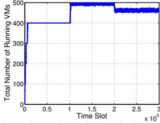
Fig. 4: The total number of running VMs in the system using OCA algorithm over all time slots.
