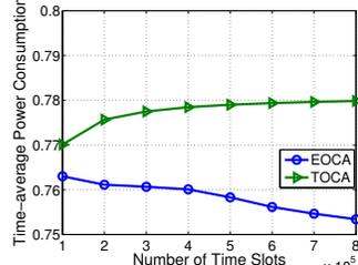
Fig. 6: Average power consumption (normalized) of servers versus the length of simulation time, with EOCA against TOCA.
