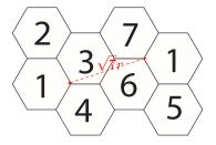
Fig. 4. Minimum distance between two points in co-coloured hexagons.
