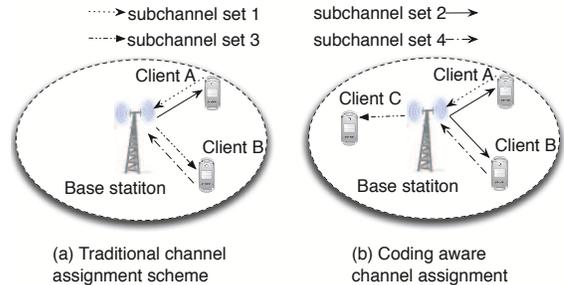
Fig. 10. The application of network coding to 802.16 OFDMA systems.
