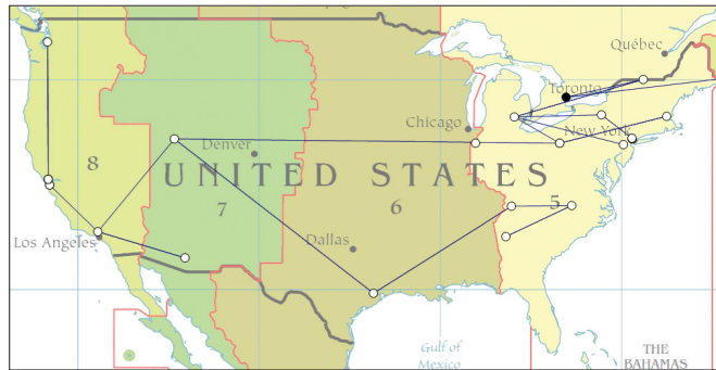
Fig. 10. The real-time wide-area topology produced by the node stress aware algorithm after 30 nodes have joined (only nodes that reside in North America have been shown, some nodes may reside in the same geographical location).
