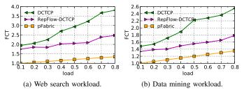
Fig. 10: Mean FCT for short flows with a 16-pod Fat-tree in NS-3. Note the different ranges of the y-axis in the plots.
