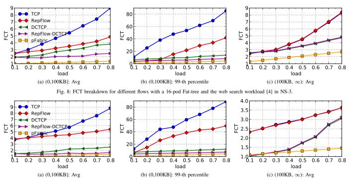
Fig. 9: FCT breakdown for different flows with a 16-pod Fat-tree and the data mining workload [15] in NS-3.
