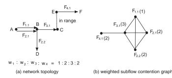
Fig. 4. Weighted subflow contention graph
