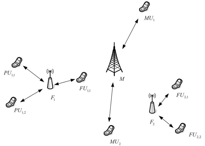
Fig. 1. System model for femtocell hybrid access.
