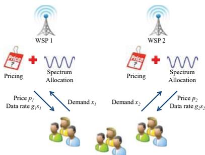
Fig. 1. Network model for the duopoly femtocell WSPs.
