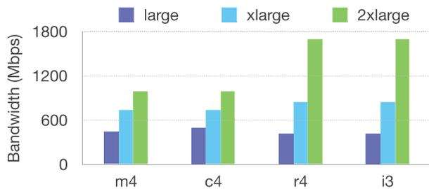
Fig. 2. Maximum bandwidth capacities across different instance families.
