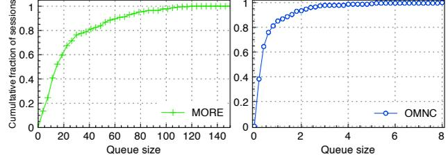
**Figure 3. The distribution of time-averaged queue size in a lossy network.**
