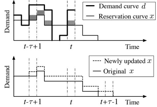
Fig. 3. Illustration of Algorithm 1. The shaded area in the top figure shows the use of an on-demand instance in the recent period. An instance is reserved at time  $t$  if the use of this on-demand instance is not well justified. The bottom figure shows the corresponding updates of the reservation curve  $x$ .
