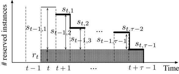
Fig. 2. Illustration of a transition into state  $\mathbf{s}_t = (s_{t,1}, \dots, s_{t,\tau-1})$  from state  $\mathbf{s}_{t-1} = (s_{t-1,1}, \dots, s_{t-1,\tau-1})$  according to (3). The shaded area stands for the  $r_t$  reservations made at time  $t$ .
