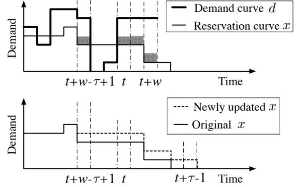
Fig. 5. Illustration of Algorithm 3. The shaded area in the top figure shows the use of an on-demand instance in  $[t + w - \tau + 1, t + w]$ . An instance is reserved at time  $t$  if the use of this on-demand instance is not well justified. The bottom figure shows the corresponding updates of the reservation curve  $x$ .
