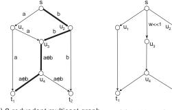
(c) 2-redundant multicast graph Throughput is doubled using network coding and alternative paths. (Dark edges form second path for t1, second path for t2 is the mirror image.)
