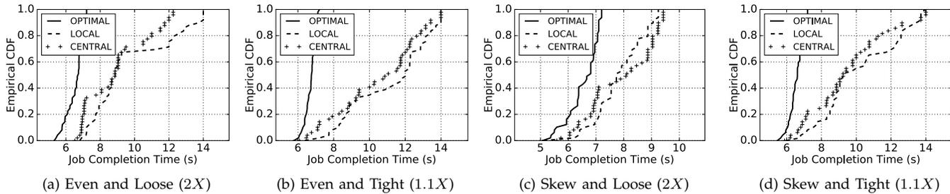
Fig. 10: The CDFs of job completion times for 50 concurrent jobs, achieved with three algorithms, with different resource availability.
