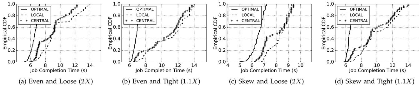
Fig. 11: The CDFs of job completion times for 100 concurrent jobs, achieved with three algorithms, with different resource availability.
