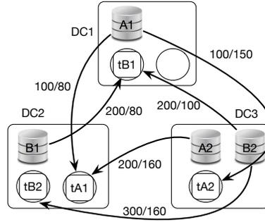
Fig. 2: A task assignment that favors the performance of job A at the cost of job B.
