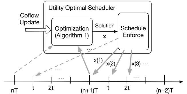
Fig. 6: An illustration of the signaling cycle of utility optimal scheduler.
