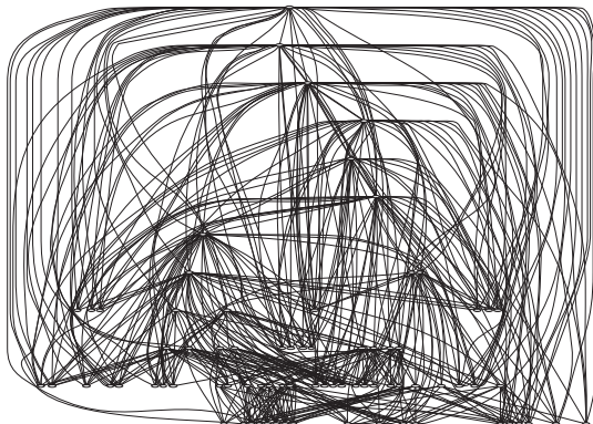
Fig. 10. Data dissemination topology in the 79-node experiment in PlanetLab, before the transitional event introducing cross traffic.
