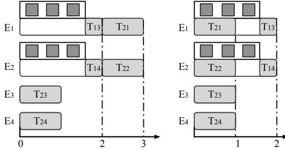
Fig. 4. Job performance without (left) and with (right) network-awareness: the completion time of Job<sub>1</sub> remains 2 time units, whereas the completion time of Job<sub>2</sub> decreases since its map stage decreases from 3 to 1 time unit.
