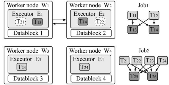
Fig. 1. A motivating example:  $T_{11}$  and  $T_{12}$  have finished and released the executors  $E_1$  and  $E_2$ .  $T_{13}$  and  $T_{14}$  are then distributed to  $E_1$  and  $E_2$ . Without network-aware scheduling, the scheduler would only launch two tasks of Job2,  $T_{23}$  and  $T_{24}$ , for now since it believes that no other executor is idle.
