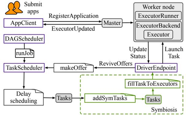
Fig. 6. *Symbiosis* on top of Spark: *Symbiosis* works as a scheduling plugin, requiring no modifications to existing application interfaces.
