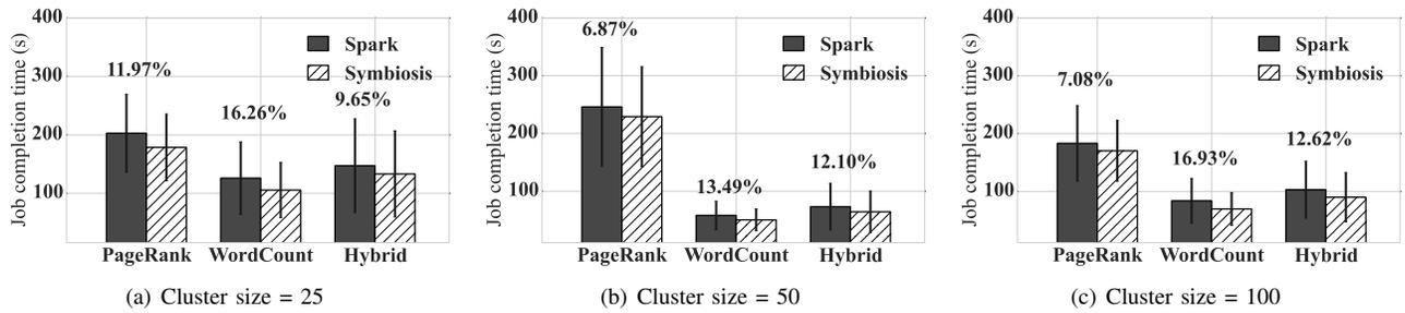
Fig. 7. Average job completion times for different workloads under three cluster sizes: jobs are expedited by more than 6% in all the experiments.
