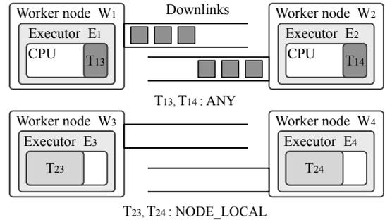
Fig. 2. In *Symbiosis*, we do not actively monitor the CPU and network utilization. We predict that  $E_1$  and  $E_2$  may experience CPU under-utilization by discovering  $T_{13}$  and  $T_{14}$  do not have any locality; we predict that  $E_3$  and  $E_4$  do not utilize the network since  $T_{23}$  and  $T_{24}$  have achieved node locality.
