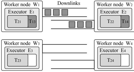
Fig. 3. Making a computation-bound task co-locate with a network-bound task corrects resource imbalance through improving CPU utilization:  $T_{21}$  and  $T_{13}$  utilize  $E_1$ 's resources, and  $T_{22}$  and  $T_{14}$  utilize  $E_2$ 's resources.
