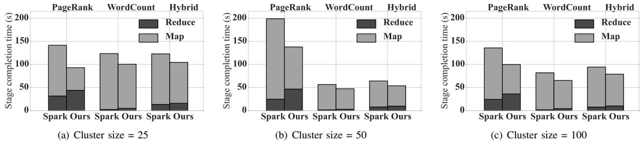
Fig. 8. The completion times of map and reduce stages for different workloads under all the three clusters. Compared with Spark, *Symbiosis* significantly speeds up the map stages due to early launching symbiotic tasks. In contrast, reduce stages are slightly slowed down due to the potential competition between a symbiotic task and the reduce task on the same executor.
