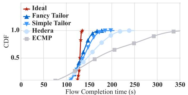
Fig. 2. The distributed functions of flow completion times within a coflow to compare Tailor with existing schemes. The coflow completion time under Simple Tailor is 205 seconds, which is 45 seconds faster than Hedera. Fancy Tailor further expedites the coflow by 30 seconds.
