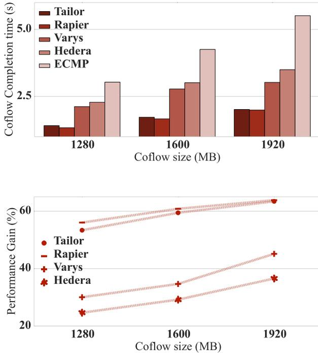
Fig. 7. Coflow performance for shuffle traffic under different coflow mechanisms: the amount of data one host sends to each receiver ranges in [20MB, 30MB]. The advantage of Tailor and Rapier over Varys is much more obvious due to the more congested network under many-to-many communication, which demonstrates the effectiveness of dynamic routing.
