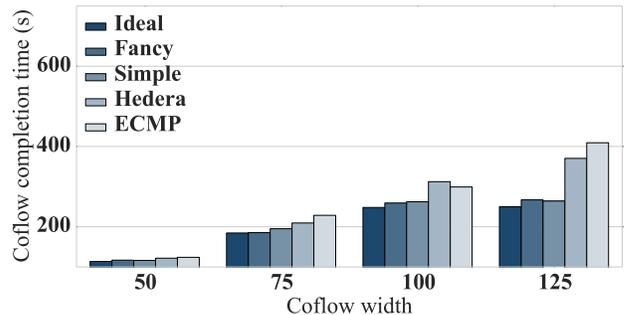
Fig. 5. Coflow performance for random traffic under different routing protocols: 80% of flows with sizes ranging from 10KB to 1MB; 10% of flows with sizes ranging from 10MB to 100MB. The advantage of *Tailor* is less significant compared with shuffle communication, since there are fewer large flows in the network.
