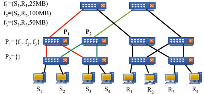
Fig. 1. A motivating example: all the links in the network are of 1 Gbps. The completion time of a coflow can be reduced if its bottleneck flow can be dynamically rerouted, e.g., routing  $f_1$  to  $P_2$ . The completion time of this coflow could be further reduced, if the currently slowest flow  $f_2$ , instead of  $f_1$ , could be rerouted from  $P_1$  to  $P_2$ .
