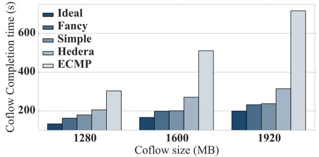
Fig. 4. Coflow performance for shuffle traffic under different routing protocols: the amount of data one host sends to each receiver ranges in [20MB, 30MB]. *Tailor* outperforms Hedera by 24.69% on average, and surpasses ECMP significantly.
