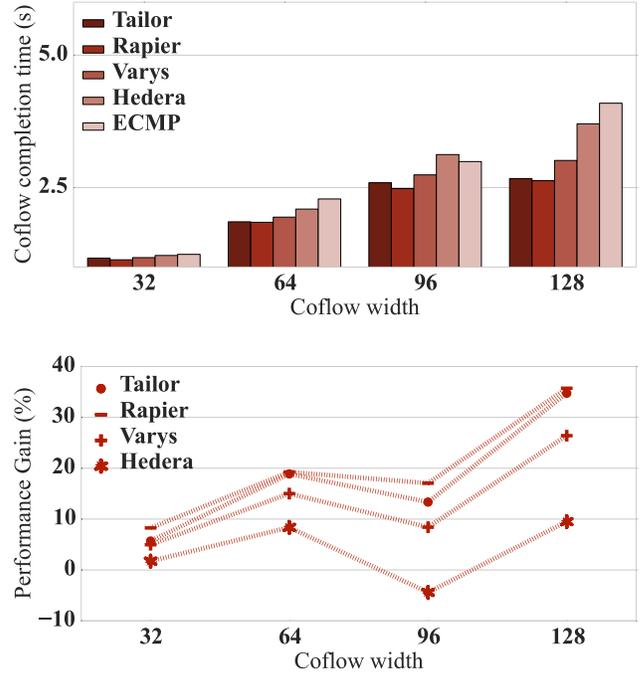
Fig. 6. Coflow performance for random traffic under different coflow schemes: the flow sizes range in [10KB, 100MB]. *Tailor* outperforms Varys in all cases, and the advantage increases with the coflow width. Tailor only achieves similar performance gain with Rapier, but it is much simpler compared to Rapier’s per-flow routing and rate limiting.
