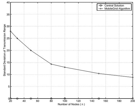
Fig. 7. Centralized Solution vs. MobileGrid (Standard Deviation of Transmission Ranges)
