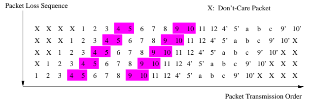
Figure 3: Packet transmission order in FEC_Retrans() ( k = 12 , h = 3 , and e = 5 )
