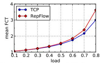
Fig. 4: Short flow mean FCT.  $k = 12$  packets, flow size distribution from the web search workload [4]. Fig. 5: Large flow mean FCT.  $k = 12$  packets, flow size distribution from the web search workload [4].
