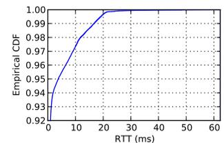
Fig. 1: CDF of RTT between two small instances in EC2 us-west-2c. Fig. 2: Long tail of the RTT distribution.
